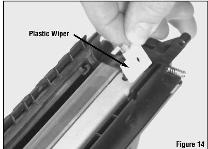
Remove the plastic wipers.
